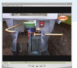
Function of the SBR wastewater treatment system Klaro
